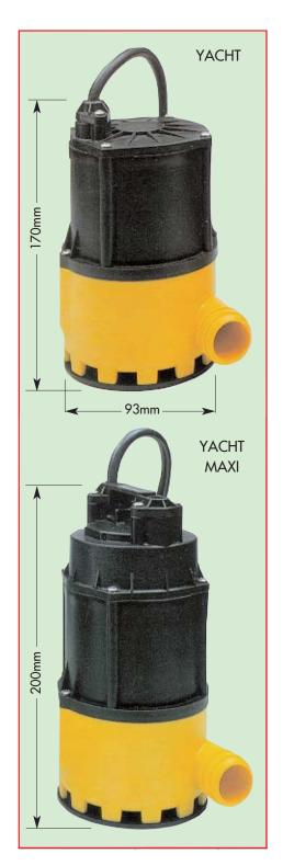
"Yacht" and "Yacht Maxi" bilge pumps are manufactured in a special crush and hydrocarbons resistant polypropylene. They are designed for easy cleaning and servicing, and feature a pull-off baseplate for access to the impeller. All pumps have a stainless steel motor shaft, with lip seals on Yacht models and mechanical seals on Yacht Maxi models. Pumps have 1" hose connectors and are supplied with 1m cable as standard.
