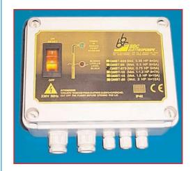
Designed for the control of 230/1/50 pumps in clean water applications such as boreholes, wells and sumps; offering protection against dry running and motor overload. Five models cover motor sizes up to a nominal 1.5kW, min 2.4 to max 12 Amps.
